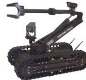
The HD2 chassis is available with a multi-axis arm attachment with a camera mast outfitted with a 360 degree PTZ camera.
