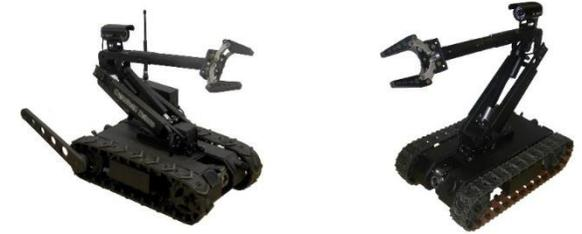
Our LT2 series of robots are also available with a multi-axis arm for EOD disposal and door opening. These are crucial to survey potentially dangerous locations.
