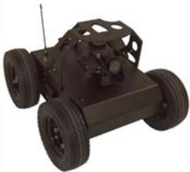
Tough, water resistant and fast, the UM4 is ideal for quick all-terrain surveillance and room clearing. The high RPM motors and six inch wheels makes this robot scale rough terrain quickly and with ease.
