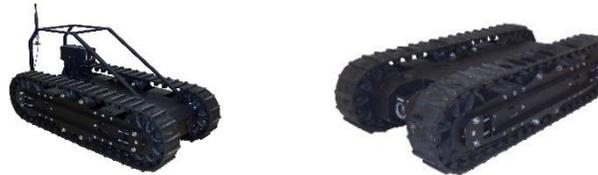
The HD2 series is our heavy duty class of robots - when power and speed are critical. Our HD2 chassis is excellent for attaching additional cameras, sensors, or to carry equipment and supplies.
