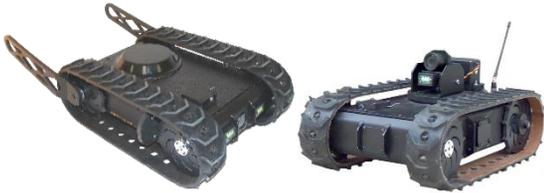
Made from heavy gauge aluminum, this lightweight and compact robot is ideal for rapid deployment, room clearing, quiet and quick surveillance, hostage negotiation, and entry into difficult areas.
